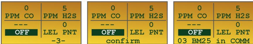
**Figure 30 : reset sequence of a group of BM 25Ws**
