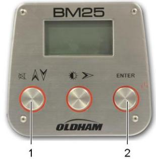
**Figure 14: press 1 and 2 to select the calibration gas**
