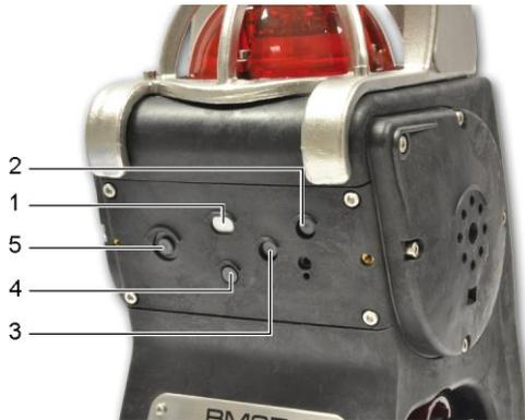
**Figure 8: sensors configuration**
